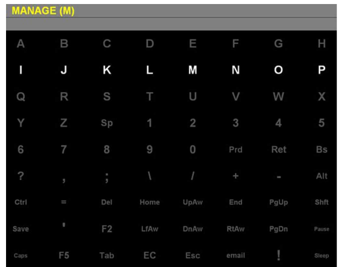
Fig. 1. Screen capture of the interface used in this study. The word to be spelled was displayed in the top gray bar followed by the current target character in parentheses. Feedback was provided by the speller displaying the character it selected below the actual target. Characters were illuminated in rows or columns, and the order was random.
